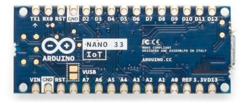
As opposed to other Arduino Nano boards, pins A4 and A5 have an internal pull-up and default to be used as an I2C bus. **So, usage as analog inputs is not recommended.**
