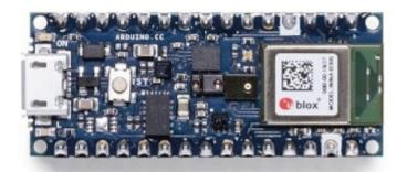
The Arduino Nano 33 BLE Sense features the same 32-bit ARM Cortex-M4 processor as the Arduino Nano 33 BLE, but also includes a bunch of onboard sensors: a 9-axis IMU, temperature, pressure, humidity, light, color, gesture sensors, and even a microphone that are managed through several specialized Arduino libraries.
