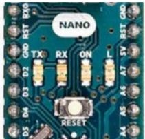
The **TX and RX LEDs** will flash when data is being transmitted via the FTDI chip and USB connection to the computer (but not for serial communication on pins 0 and 1).
