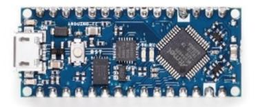
The Arduino Nano Every is one of the newer, more powerful Arduino Nano boards. It uses the ATmega4809 microcontroller and is the cheapest Arduino board you can buy!
